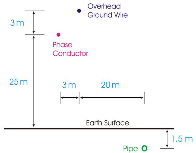
Fig. 2. Cross-section of the corridor shared by a transmission line and a pipeline.
