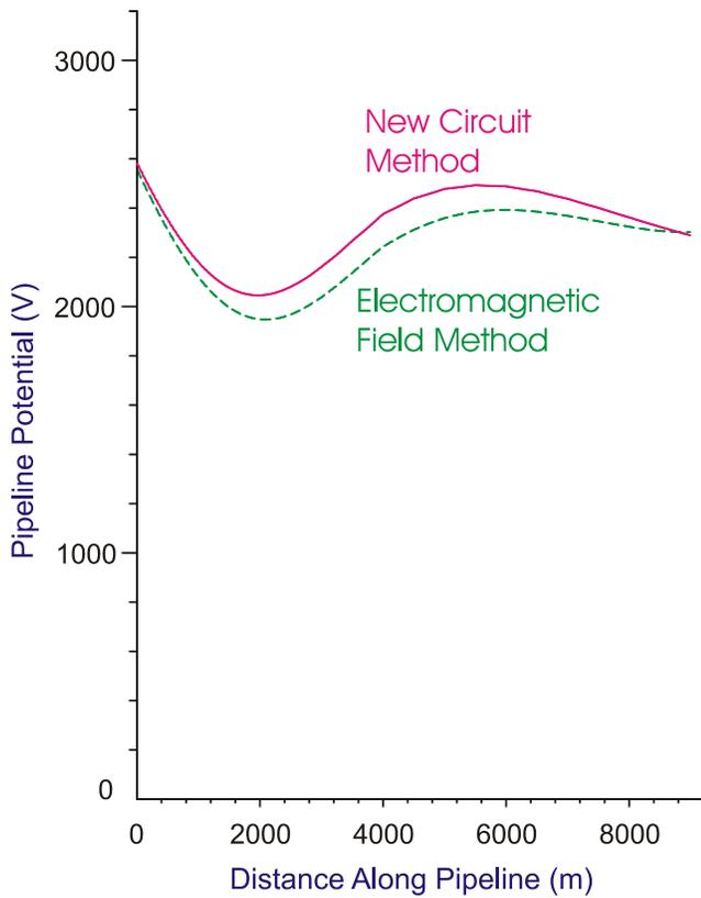
Fig. 8. Pipeline potentials computed using the electromagnetic field method and the new circuit method.
