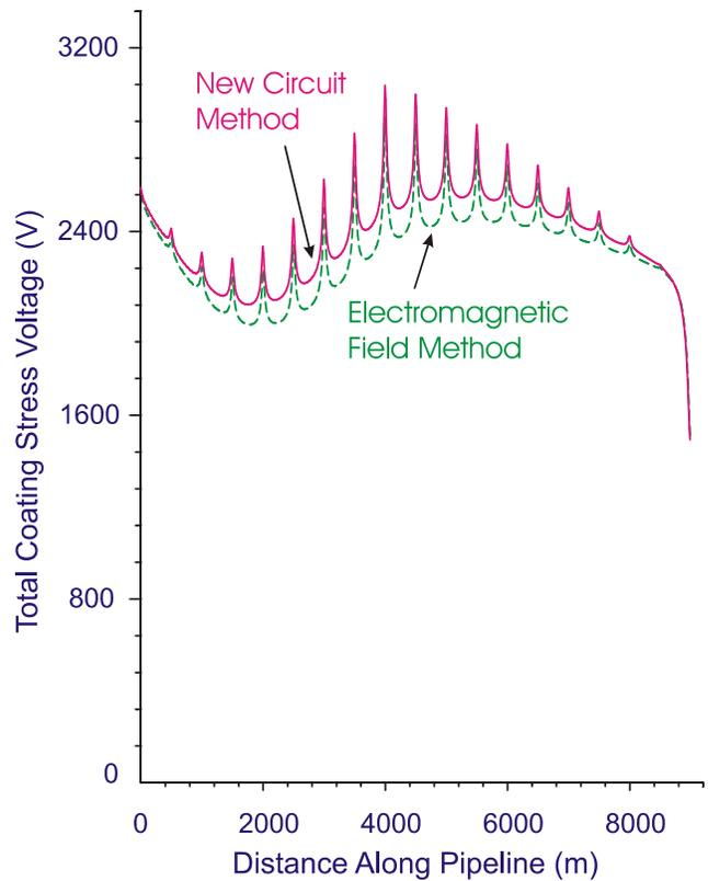
Fig. 10. Total coating stress voltages computed using the electromagnetic field method and the new circuit method.
