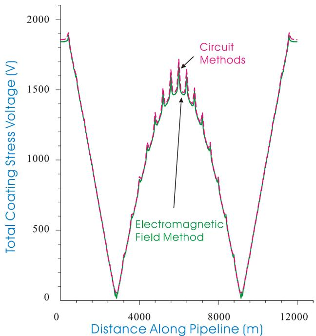
Fig. 4. Total coating stress voltage computed using the circuit methods and the electromagnetic field method.
