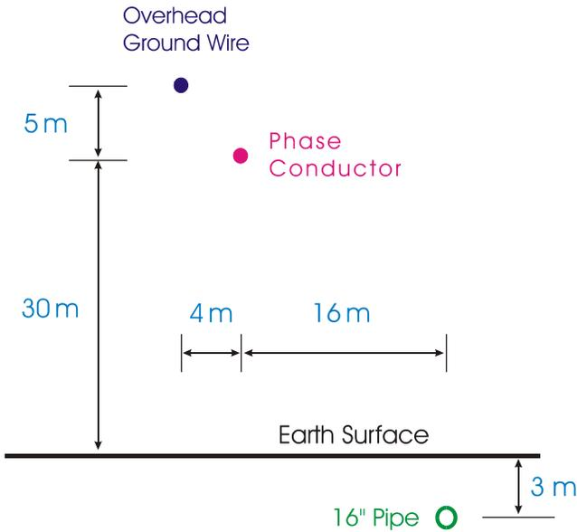
Fig. 6. Cross-section of the common corridor shared by a transmission line and a pipeline connected to a grounding grid of the transmission line system.
