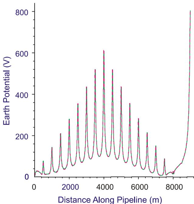
Fig. 9. Earth potentials along the pipeline computed using the electromagnetic field method and the new circuit method.
