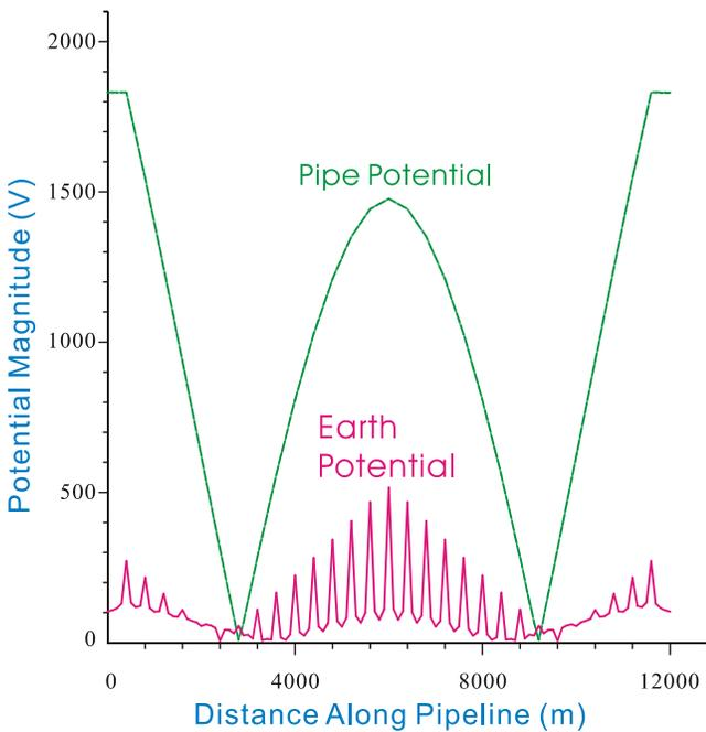
Fig. 3. Pipeline potential and earth potential computed using the conventional circuit method (CCM) followed by a grounding analysis.
