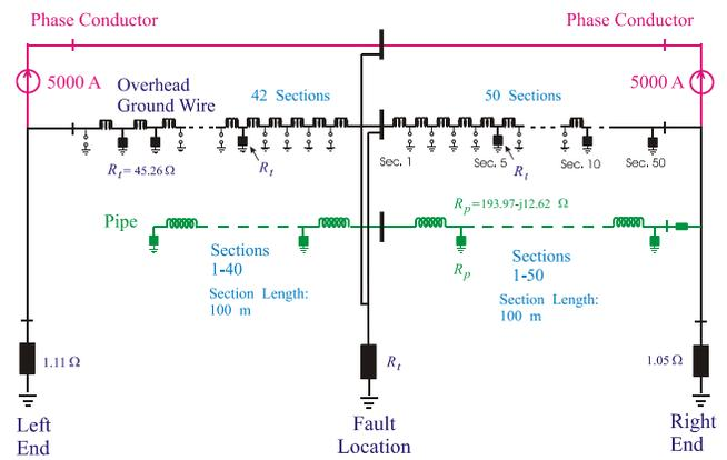
Fig. 7. Circuit model for the common corridor shared by a transmission line and a pipeline.
