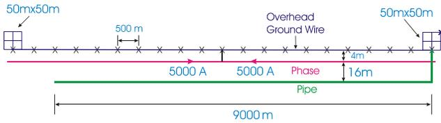
Fig. 5. Plan view of the common corridor shared by a transmission line and a pipeline connected to a grounding grid of the transmission line system.
