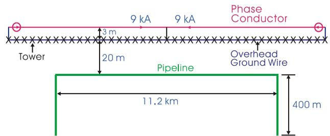
Fig. 1. Plan view of the corridor shared by a transmission line and a pipeline.
